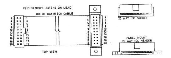
CONSTRUCTING RIBBON CABLE EXTENSION LEAD :-
